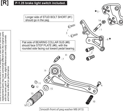
should face pedal bearing, with the
