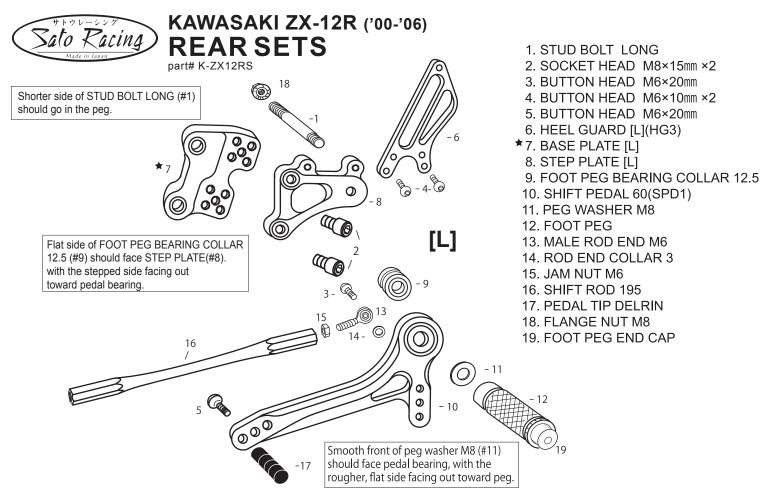
**XADJUST THE STOCK CHANGE ARM WHEN INSTALLING SATO REAR SETS.**
