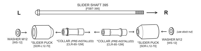
\* Slider Puck and Collar are sold with together as a single part, with the Collar pre-installed inside the Slider Puck.
