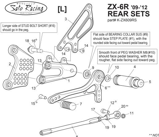
**%ADJUST THE STOCK CHANGE ARM WHEN INSTALLING SATO REAR SETS.**
