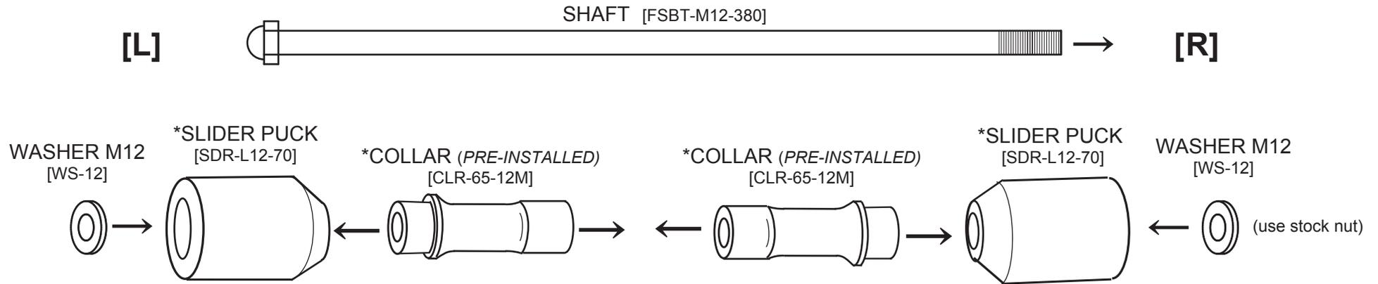
\* Slider Puck and Collar are sold with together as a single part, with the Collar pre-installed inside the Slider Puck.
