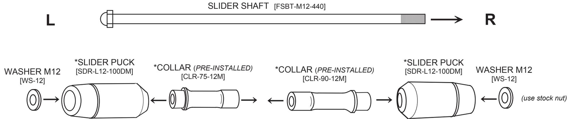
\* Slider Puck and Collar are sold with together as a single part, with the Collar pre-installed inside the Slider Puck.
