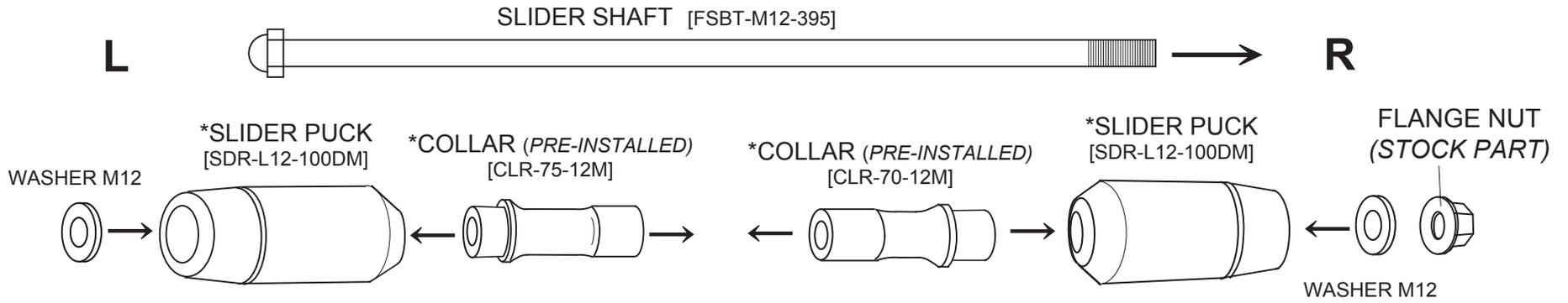
\* NOTE: Collar is pre-installed inside the Slider Puck. When ordering a replacement Slider Puck, please mention the Collar part number.
