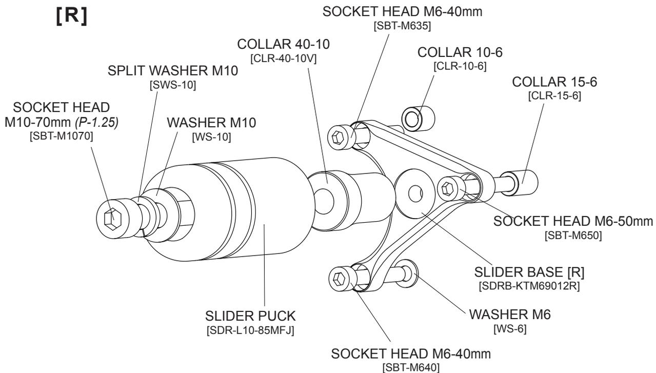
\* NOTE: Some 2012-15 KTM 690 Duke were assembled with the threaded end of the engine mount bolt on the right side instead of the left side as originally spec'd. In these cases, the bolt will need to be removed and flipped the opposite direction to install these Frame Sliders.
