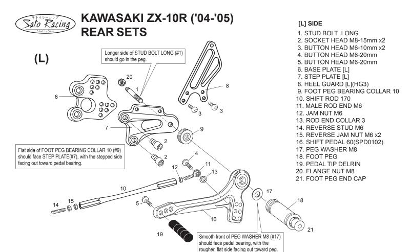
**X ADJUST THE STOCK CHANGE ARM WHEN INSTALLING SATO REAR SETS.**
