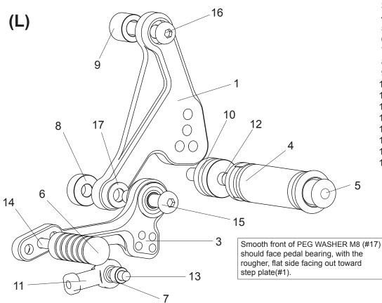
1. STEP PLATE [L] 3. SHIFT PEDAL(SPD10) 4. FOOT PEG 5. FOOT PEG END CAP 6. PEDAL TIP 7. ROD END COLLAR 6(GD) 8. BASE PLATE COLLAR 8(BK) 9. COLLAR 14-10(BK) 10. FOOT PEG COLLAR 15 11. FEMALE ROD END M6 12. STUD BOLT M8-40mm 13. FLANGE HEAD M6-25mm 14. BUTTON HEAD M6-20mm 15. BUTTON HEAD M8-45mm 16. BUTTON HEAD M8-55mm 17. PEG WASHER M8
